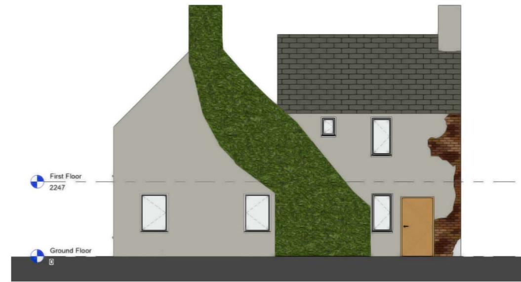
Fig13: Condition East Elevation (Author, 2021)
