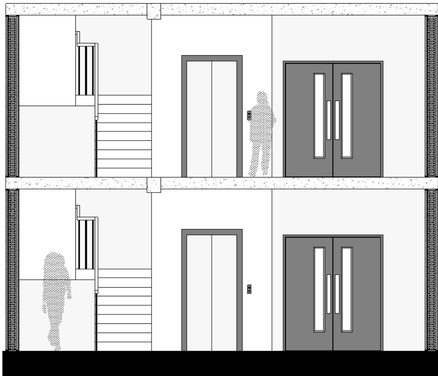
Fig101 - Enlarged Fire Core Section (Author, 2021)
