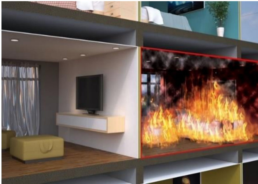
Fig10 - Fire Compartmentation (Promat, 2020)
